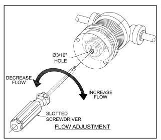
The water flow can be adjusted using a slotted narrow blade screwdriver and turning clockwise to increase flow and counterclockwise to decrease flow.
